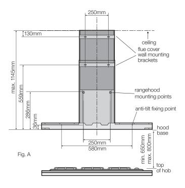
3. Install flue cover wall mounting brackets with suitable fixings. Install suitable screws for rangehood mounting points (to support a total weight of 30kg) to the wall as marked (Fig. B).
