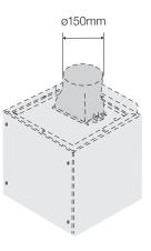
NOTE: The fan housing flue transition duct is 150mm in diameter. (See page 10 for optional ducting accessories).
