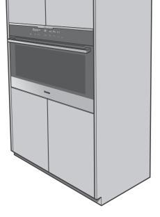
For the best integration within a kitchen, install this appliance in a cupboard that gives a flush fit with the surrounding cupboard fronts. A recess of 20mm is ideal.
