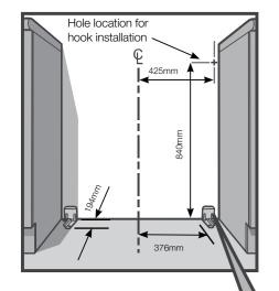
Measurements are to be adjusted to account for the thickness of any skirting board or tiles coming between the back of the appliance and the wall
