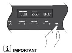
At the beginning of Pyrolytic cleaning the door will automatically lock will appear on the display. During the Pyrolytic cleaning cycle there may be some burn off odours. It is advised to keep the room well ventilated during this cycle. The door will only unlock when the oven has cooled to a safe temperature. Turning the function off will not unlock the door. This will only happen when safe temperatures are reached.
