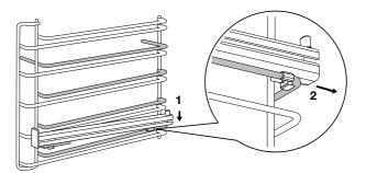
3. Push slide front clip over wire until secured.
