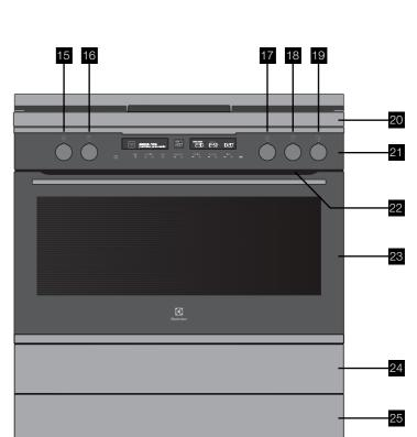
Rapid burner control 15 Semi rapid burner control 19 20 Gas hob Auxiliary burner control Wok burner control 21 Control panel (see above) 22 Exhaust air outlet 18 Semi rapid burner control
