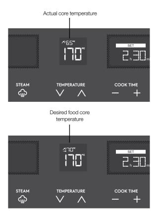
NOTE: The end time/cook time function cannot be set whilst using the Food Probe function.
