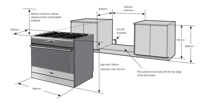
The freestanding type installation uses the appliance as supplied, and can be fitted in between cabinets, with cabinets on one side or without adjacent cabinets. There is no clearance requirement to adjacent side cabinets.
