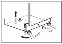
To adjust the rear height of the appliance, turn the middle screw counterclockwise.
