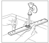
4. To install the spray arm back, press the spray arm upwards and simultaneously turn it counterclockwise until it locks into place.
