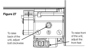
f. Adjust the leg levellers (Fig. 28) so that they touch the ground and can't be rotated further by bare hands. This will stop the refrigerator rolling forward when opening the doors.
