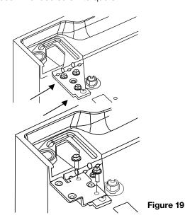
Assemble the Replacement Top Hinge Cover to the Top Hinge using the screw removed from factory fitted Top Hinge Cover. (Fig. 20)
