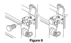
Attach Clip Trim Bottom to the inside of each leveller assembly using screws 9H
