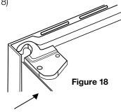
Remove the two screws shown. Attach the bracket to the top hinge using the removed screws.
