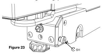
b. Locate slot in right hand side trim over shoulder screw
