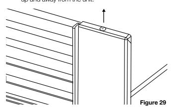
h. Drill dia 3.2mm pilot holes on the cabinetry and secure the Top Trim to the cabinetry using two screws each on left and right ends.
