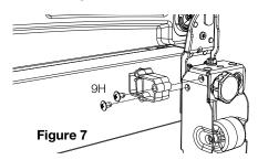
e. Repeat the procedure to fix the other levelling system to other side of the refrigerator.
