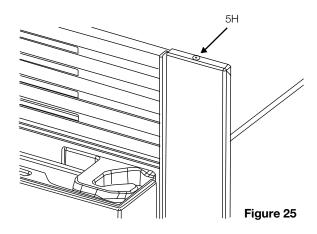
d. Assemble the left hand side trim to the appliance using the same method.
