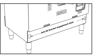
The following steps must be followed to ensure the correct installation of anti-tilt brackets and the stability of the appliances.
