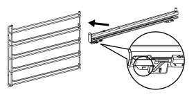
2. The shaded wires indicate the wire the slide can be mounted on. Fit slide rear clips to the rear of wire at an angle as shown below.
