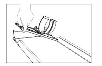
3 Make sure both clip modules are in the same orientation after installation.
