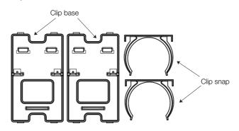
1 Assemble the clip snap onto the base.
