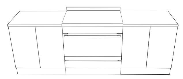
The slot-in type installation use the appliance as supplied. The appliance can be mounted on a plinth. This enables a continous cupboard kickboard to be installed, giving a more intergrated appearance. There is no clearance requirement between oven and adjacent side cabinets.
