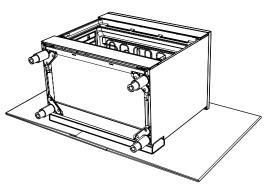
Adjust the height of the screw-in feet to make sure the hob surface is 10mm above the bench when appliance is upright.
