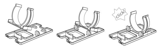
2 Press in both assembled clip modules into the kick panel in the orientation as shown below.
