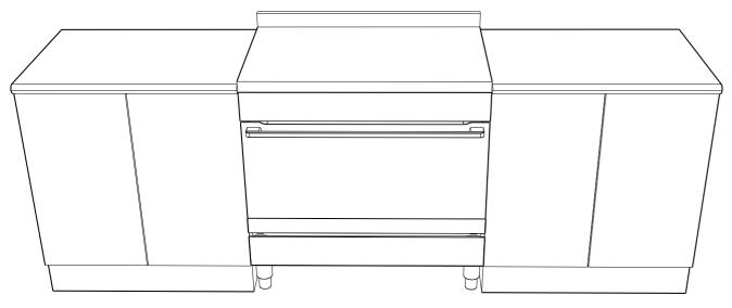
The freestanding type installation requires four screwin feet to be installed before it can be fitted in between cabinets, with cabinets on one side or without adjacent cabinets. There is no clearance requirement to adjacent side cabinets. Four screw-in feets are supplied with the appliance and can be found in the accessories pack in the oven.
