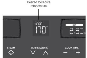
NOTE: The end time/cook time function cannot be set whilst using the Food Probe function.
