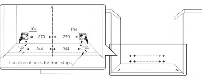
Measurements are to be adjusted to account for the thickness of any skirting board or tiles coming between the back of the appliance and the wall
