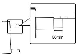
For a 900mm height kitchen bench top, adjust the lower half of the feet to measure 50mm as shown in the illustration.
