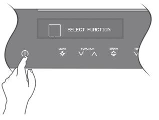
2 Select a cooking function by pressing the  $\land$  function or  $\lor$  function as many times as necessary until the desired function appears.
