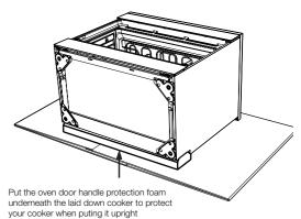
Install the four supplied feet via the four installation points. Make sure that each foot is securely fastened.
