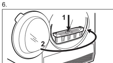
1) If necessary remove fluff from the filter socket and gasket. You can use a vacuum cleaner.
