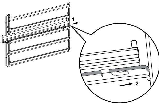
Push slide front clip over wire until secured
