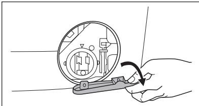
2. Place a suitable water container below the recess of the drain pump to collect the water that flows out. Press the two levers and pull forward the drainage duct to let the water flow out.
