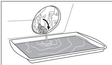
3. When the container is full of water, put the drainage duct back again and empty the container. Do step 2, 3 again and again until no more water flows out from the drain pump.
