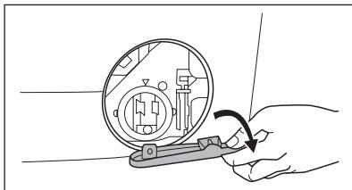
2. Place a suitable water container below the recess of the drain pump to collect the water that flows out. Press the two levers and pull forward the drainage duct to let the water flow out.
