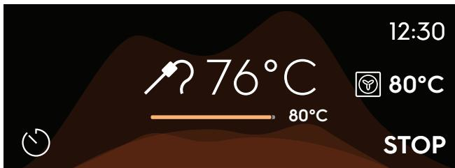
*NOTE: The Food Sensor/probe temperature will not be displayed until the oven is at the desired temperature. Once the oven is at the desired temperature, the Food Sensor/probe temperature will cycle between the desired food core temperature and the actual food core temperature.*
