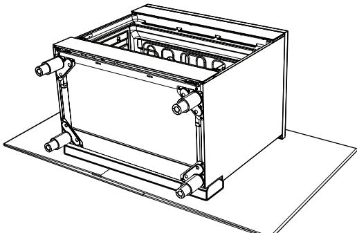
Adjust the height of the screw-in feet to make sure the hob surface is 10mm above the bench when appliance is upright.
