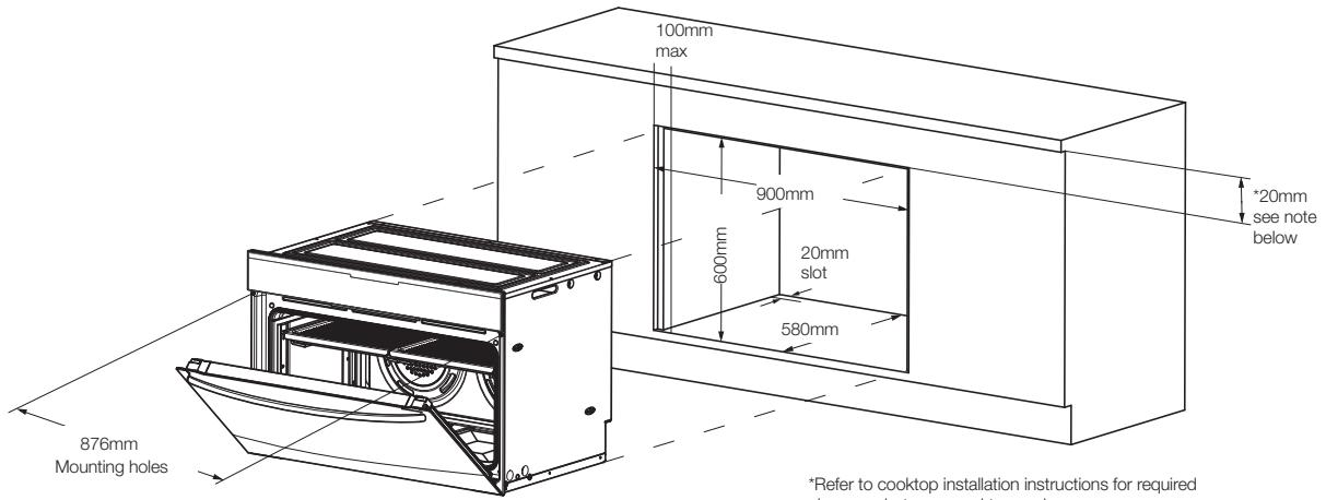
*NOTE: If a powerpoint is fitted it must be accessible with the appliance installed.*
