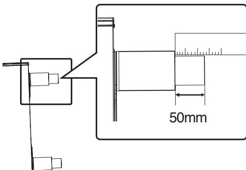
For a 900mm height kitchen bench top, adjust the lower half of the feet to measure 50mm as shown in the illustration.
