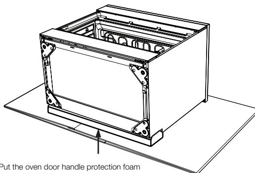
Put the oven door handle protection foam underneath the laid down cooker to protect your cooker when putting it upright
