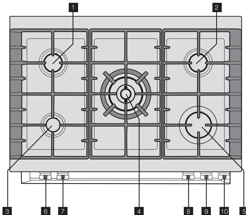
**1** 9.0MJ/h Medium heat burners. Used for simmering with mid-sized cookware.
